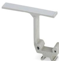
Group marking label, can be snapped into terminal center for screw, spring-cage, push-in, and fast connection terminal blocks, can be labeled with a 24 x 4 mm label or manually using B-STIFT, in the foot part with ZB 5
