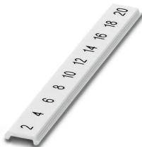
Zack Marker strip, flat, Strip, white, labeled, printed horizontally: consecutive even numbers 2 ... 20, 22 ... 40, etc. up to 82 ... 100, mounting type: snapped, for terminal block width: 5 mm, lettering field size: 5.15 x 5.15 mm, Number of individual labels: 10
