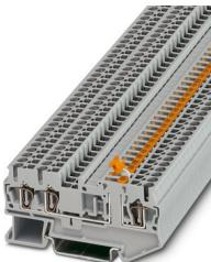
Knife-disconnect terminal block, nom. voltage: 400 V, nominal current: 20 A, 1 level, connection method: Spring-cage connection, Rated cross section: 2.5 mm<sup>2</sup>, cross section: 0.08 mm<sup>2</sup> - 4 mm<sup>2</sup>, mounting: NS 35/7,5, NS 35/15, color: gray
