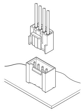
This is VH connector high box type, with 21.3 mm mounting height (single circuit: 18.6 mm) and with 9.2 mm thickness (single circuit: 8 mm). This connector exhibits the stable electric connection to the condition such as the vibration, the prying, the microcurrent and micro-voltage circuit.
