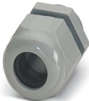
Cable gland, material for screw connection: PA, external cable diameter 22 mm ... 32 mm, shielding: no, connecting thread: M40 x 1.5, color: silver-grey RAL 7001
