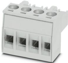
PCB connector, nominal cross section: 2.5 mm<sup>2</sup>, color: light grey, nominal current: 16 A, rated voltage (III/2): 320 V, contact surface: Tin, contact connection type: Socket, number of rows: 1, number of positions: 4, product range: MSTBT 2,5 HC/..-STP, pitch: 5 mm, connection method: Screw connection with tension sleeve, conductor/PCB connection direction: 0 °, locking clip: - Locking clip, plug-in system: COMBICON MSTB 2,5 HC, locking: without, mounting: without
