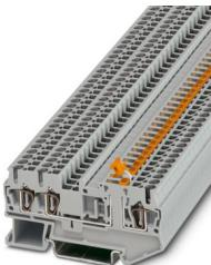
Knife-disconnect terminal block, nom. voltage: 400 V, nominal current: 20 A, 1 level, connection method: Spring-cage connection, Rated cross section: 2.5 mm<sup>2</sup>, cross section: 0.08 mm<sup>2</sup> - 4 mm<sup>2</sup>, mounting: NS 35/7,5, NS 35/15, color: gray
