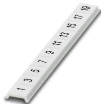
Zack Marker strip, flat, Strip, white, labeled, printed horizontally: Odd numbers 1 - 19, 21 - 39, etc. up to 81 - 99, mounting type: snapped, for terminal block width: 5 mm, lettering field size: 5.15 x 5.15 mm, Number of individual labels: 10
