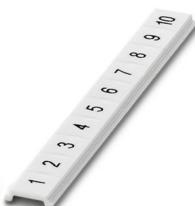
Zack Marker strip, flat, Strip, white, labeled, printed horizontally: consecutive numbers 1 ... 10, 11 ... 20, etc. up to 491 ... 500, mounting type: snapped, for terminal block width: 5 mm, lettering field size: 5.15 x 5.15 mm, Number of individual labels: 10
