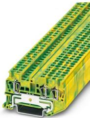
Ground terminal, number of connections: 3, connection method: Spring-cage connection, cross section: 0.08 mm<sup>2</sup> - 4 mm<sup>2</sup>, mounting type: NS 35/7,5, NS 35/15, color: green-yellow
