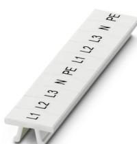
Zack marker strip, Strip, white, labeled, horizontal: L1, L2, L3, N, PE, L1, L2, L3, N, PE, mounting type: snapped, for terminal block width: 5.2 mm, lettering field size: 5.15 x 10.5 mm, Number of individual labels: 10
