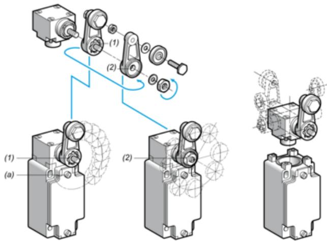
(1) 5° steps throughout 360° / Tightening torque (Min : 1) (Max : 1.5)
