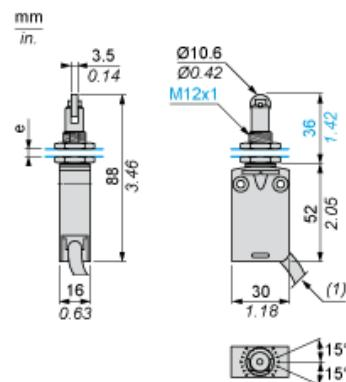
(1) External diameter of cable 7.5 mm.
