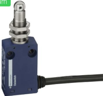
**Limit switch, Limit switches XC Standard, XCMN, M12 steel roller plunger, 1NC+1 NO, snap, 1 m**
