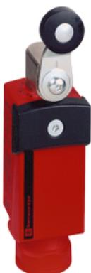
**Safety limit switch, Telemecanique Safety switches XCS, plastic, rotary lever, 2NC+1 NO, 1entry tapped M20 x 1.5**
