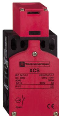
**Safety switch, Telemecanique Safety switches XCS, plastic XCSTA, 2 NC + 1 NO, slow break, 2 entries tappedM16**
